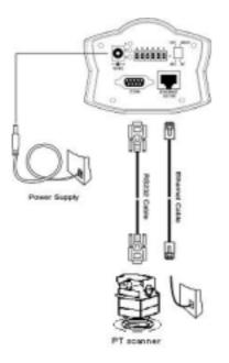
Shut down all the peripheral devices prior to connection. Connect the supplied cables from NetworKam to related devices according to the above diagram. Note that the power adaptor must be kept unplugged until other cables are firmly connected.
